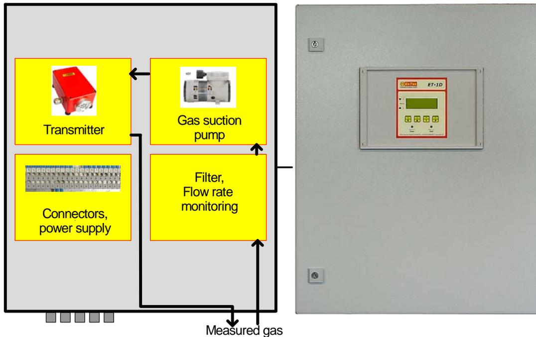
Description : Integral Measuring Concept: Sampling and conditioning of measured gas as well as transmitters and evaluation combined in one wall mounted housing.
