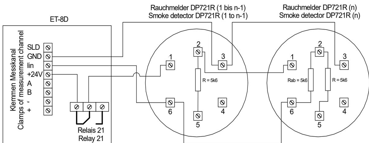
Inside the ET-8D Relay K21 has to be included into wiring. For several smoke detector lines the supplies (clamp 1) should all be done from the mid contact ("Common") of Relay K21. In all smoke detectors resistors ( $R = 5.6 \text{ k}\Omega$ ) have to be installed between clamps 2 and 5. For the last smoke detector of each line and additional terminating resistor ( $R_{ab} = 5.6 \text{ k}\Omega$ ) has to be installed additionally between clamps 2 and 6.
