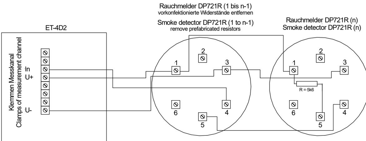
In all smoke detectors resistors ( $R = 5.6\text{ k}\Omega$ ) have to be installed according to the figures. The resistors are included in the red protection caps or already installed.
