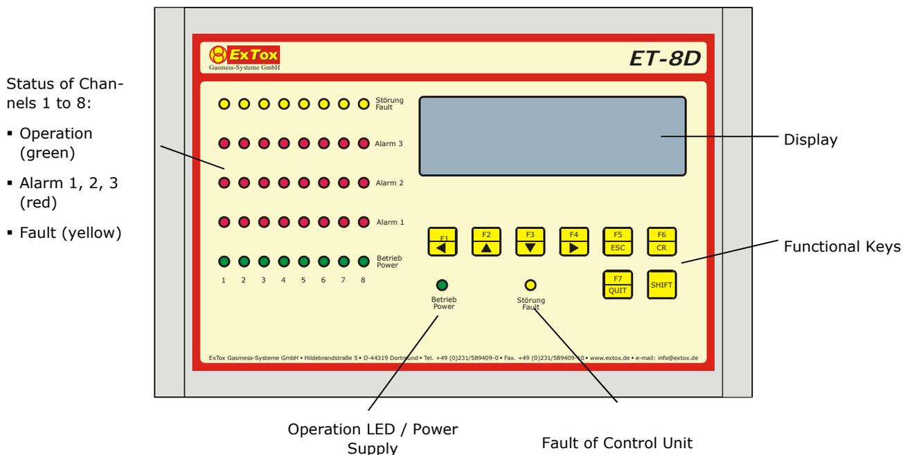
The display indication and the assignment of the functional keys F1 to F8 varies in the different operation modes of the ET-8D. The corresponding assignment of the functional keys is indicated in the line at the bottom of the graphic display.
