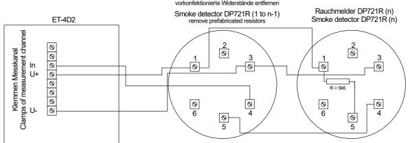
In all smoke detectors resistors (R = 5.6 k $\Omega$ ) have to be installed according to the figures. The resistors are included in the red protection caps or already installed.
