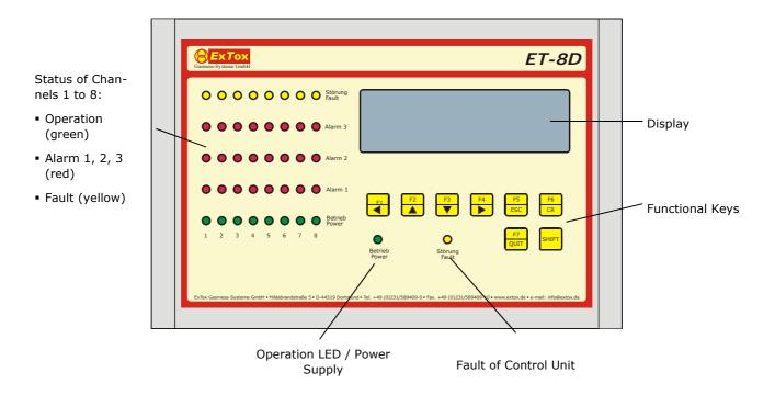
The display indication and the assignment of the functional keys F1 to F8 varies in the different operation modes of the ET-8D. The corresponding assignment of the functional keys is indicated in the line at the bottom of the graphic display.
