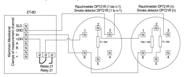
Inside the ET-8D Relay K21 has to be included into wiring. For several smoke detector lines the supplies (clamp 1) should all be done from the mid contact ("Common") of Relay K21. In all smoke detectors resistors (R = 5.6 k $\Omega$ ) have to be installed between clamps 2 and 5. For the last smoke detector of each line and additional terminating resistor (R<sub>ab</sub> = 5.6 k $\Omega$ ) has to be installed additionally between clamps 2 and 6.
